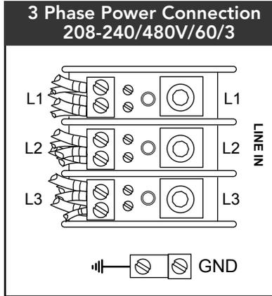
Fig. 12 - 3PH terminal block
