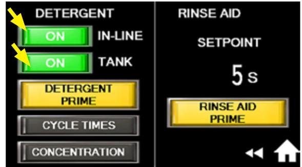
Fig. 36 - In-line and Tank sensor selected.
