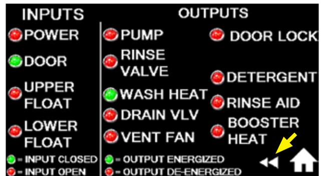
Fig. 54 - I/O SCREEN - Component status
