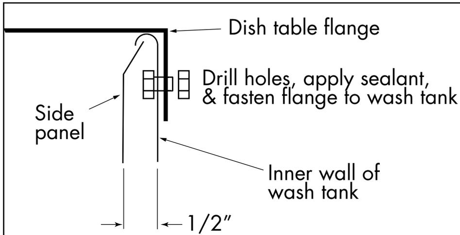
Fig. 2 - Dish table installation (if required)
