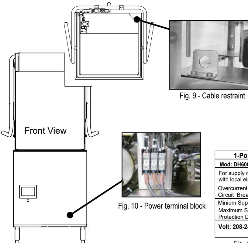
Fig. 9 - Cable restraint
