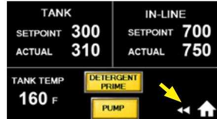
Fig. 39c - Tank and In-line Sensors ON
