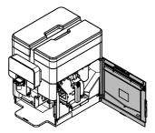
Remove the brew group by pulling it by the handle and pressing the «PRESS» button.
