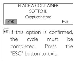
Place an empty container of at least I litre capacity under the dispensing spout and press the "OK" button to confirm. The machine performs a Cappuccinatore standard clean cycle.
