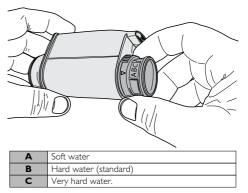
Immerse the water filter vertically in cold water (with the opening positioned upwards) and gently press its sides to let the air bubbles out.
