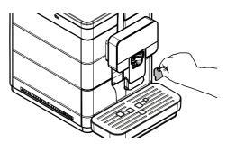
Insert the Cappuccinatore into its seat until it locks into place. Check that it cannot be pulled out.
