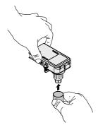
Insert the tube on the left-hand side of the fitting.
