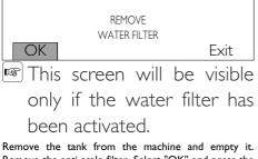
Remove the anti-scale filter. Select "OK" and press the "OK" button. The following screen is displayed:
