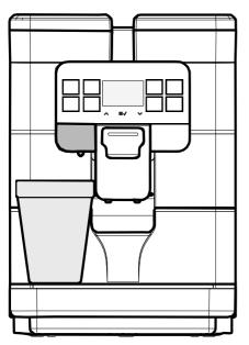
Press the "Hot Water" button to start dispensing HOT WATER.
