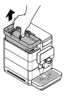
Use a non-abrasive detergent to wash it, rinse with fresh water and dry carefully.
