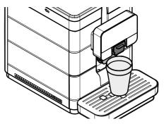
Press the "Coffee" button to start brewing. The machine starts brewing coffee from the dispensing spout. Wait until brewing has been completed and empty the container. Repeat the brewing process 3 times.
