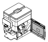
Remove the brew group by pulling it by the handle and pressing the «PRESS» button. The brew group must be washed with lukewarm water only. Do not use any detergent.
