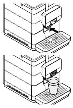
Before brewing any product and/or when bringing the dispensing At first start-up, the desired display language of the messages must be selected and stored. spout back to its normal position, ensure that it is correctly positioned. This can be evidenced by the CLICK indicating correct positioning.
