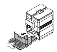
After emptying it put the drip tray back into place. Select "OK" and press the "OK" button. The following screen is displayed:
