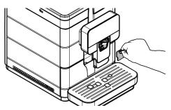
Insert the Cappuccinatore into its seat until it locks into place. Check that it cannot be pulled out.
