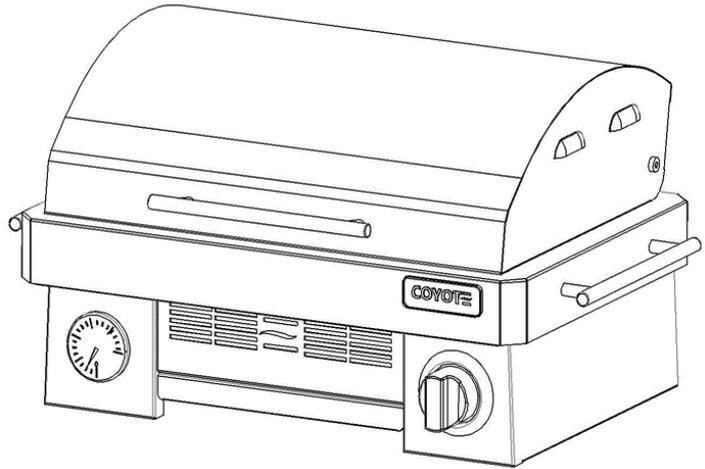
3. Depress and rotate the knob corresponding to the burner counter-clockwise to the "High" position.
