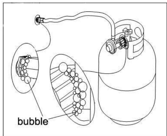
7. If no rushing sound, brush soapy solution onto areas where bubbles are shown in LP tank (see picture).
