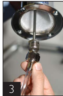
3 Thread beer line connector to draft arm and secure draft arm to cabinet with rubber gasket under the draft arm.
