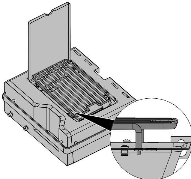
**Cooking Grid Placement:** The cooking grid can be placed at two different heights. The lower height is for use with pots or pans. The higher position is to be used when searing meats. Ensure the burner is off and the grid is cool to the touch before changing between the two heights. The grid must be at the lower height in order to close the lid.
