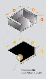
Allow minimum of 4.25" clearance from the grill's rear edge and 2.625" from the cutout to the backsplash to allow hood to fully open.
