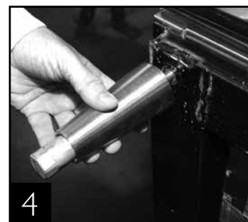
4 Thread leg into cabinet bottom frame rail.
