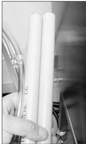
Chemical Pick-up Tubes, stiffener tubes & line strainers.
