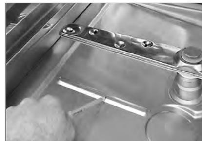
Proper Water Level in the Wash Tank.
